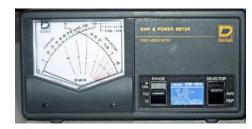
An SWR meter can be calibrated to give average or PEP readings under operating conditions or a separate power meter may be available for use under test conditions
