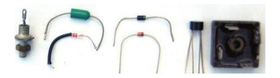
A diode is a device which conducts electricity in one direction only
